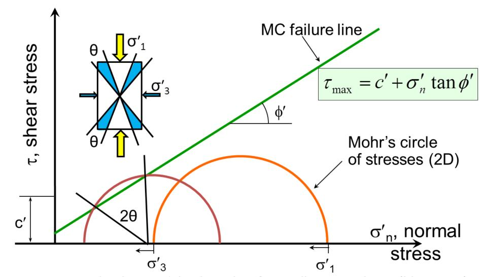
Increasing p and reducing  $\sigma'_n$  leads to slip of critically oriented joint (blue areas).
