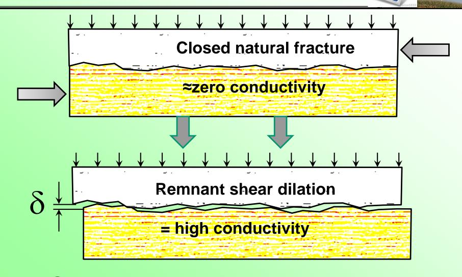
**Shear Dilation in Hydroshearing**
