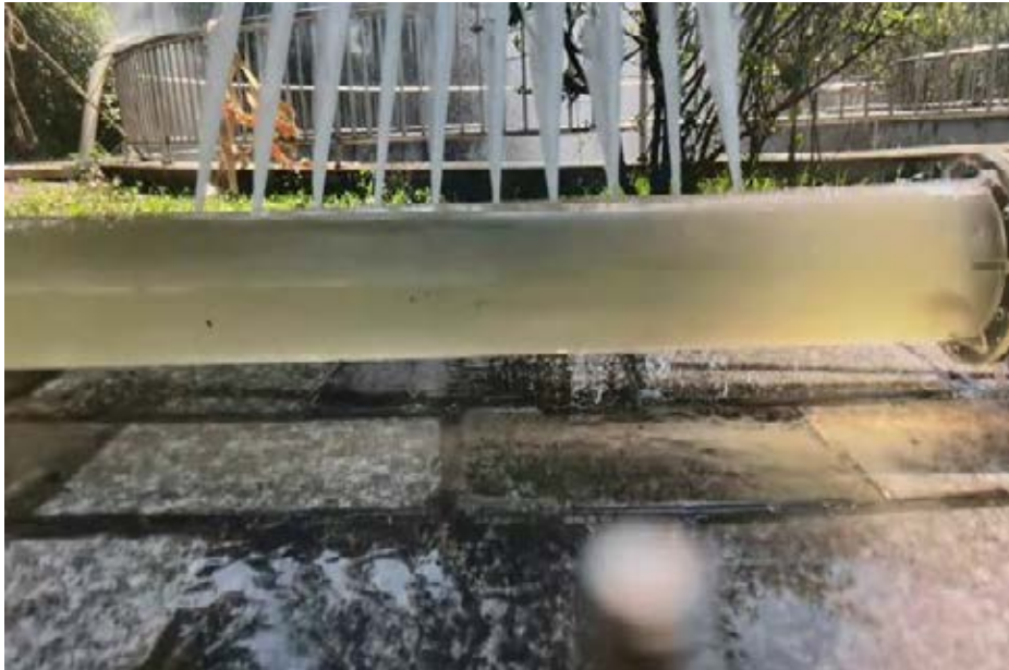
The TPF ball is prone to sink to the bottom and fails to achieve effective blocking
