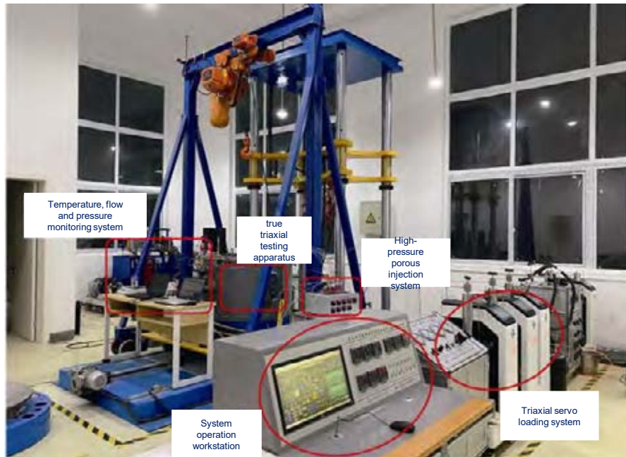
A true triaxial experimental system integrating drilling, fracturing and production
